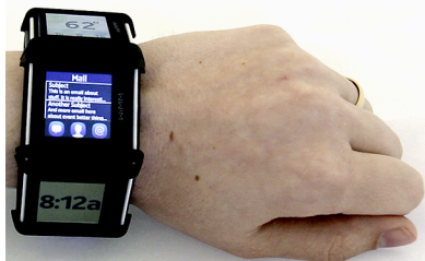
Figure 8. Facet is a multi-display bracelet consisting of independent touch-sensitive segments.
