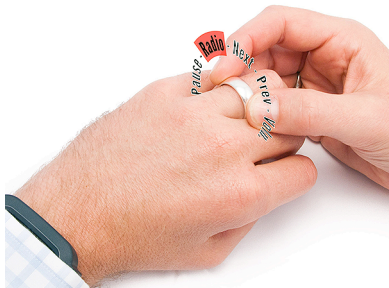
Figure 7. Nanya is a magnetic ring allowing simple input actions such as twist to select and slide to click.
