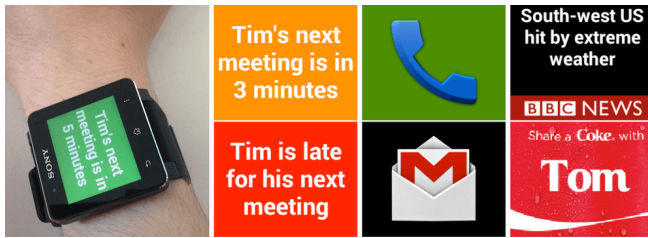
Figure 4. Examples of the displays of each of the three probes. Left: the meeting reminder display as shown on a Sony SmartWatch 2. Note that the text is upside-down to the wearer, but upright for the glancer. Other images, from left to right: the wearer’s content, showing two further stages of the meeting reminder; a glancer’s content, showing a call alert from a person marked as important (top), and a normal email alert (bottom); and, public content, showing a news headline, and an advert.
