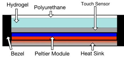
**Figure 4.** This figure illustrates the layers of the prototype used to activate the gel. Here a Peltier module is set to cool the gel (blue side).
