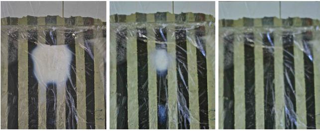
**Figure 6.** Hydrogel states as temperature is changed, Left: The gel is at its hardest, feeling like an oil-based paint. Centre: The gel is softer and thinned out, feeling more like an acrylic-based paint. Right: The gel is now at its softest after being fully thinned out, and feels more like a water-based paint.
