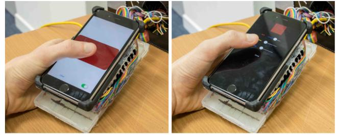
**Figure 7.** The GUI displayed on the phone. On the left is the menu to select the initial colour. On the right we see the chosen colour now in the centre pot, which activates the gel in that area on the back of the device.
