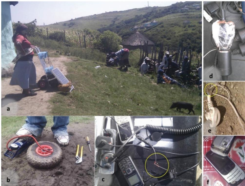
Fig. 4. Final version of Ridge Station moved further from the rondaval than normal because of a meeting - a weakened panel is not attached to the cart (a); broken components at Ridge (b); repairing a tyre during a break in the rain in the wet season (c). Examples at Ngcobo of: operator-repaired charger (d); plug to Headman's generator (e); and, inhabitants' phones (f).
