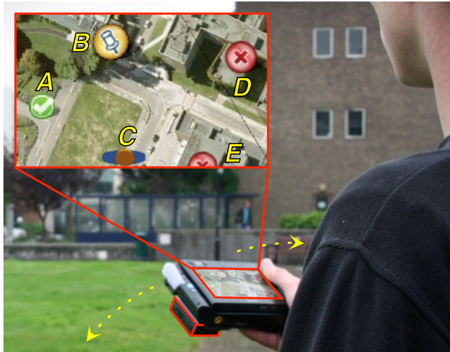
FIGURE 4.4: The visual browsing comparison system, showing the on-screen display (inset). Point A has previously been selected, point B is currently being pointed at by the user and is activated. Point C represents the user at their current position. The two remaining points, D and E, have not yet been visited.
