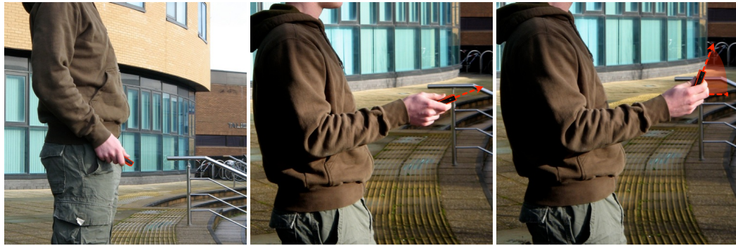
FIGURE 3.1: Specifying the distance of a selection. Left to right: the user takes the device (highlighted in each image) from their side, points in the direction of their selection and then tilts back to approximate the target’s distance. The angle of tilt (shaded in the rightmost image) specifies the distance being selected.
