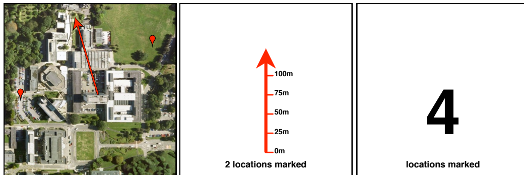
FIGURE 3.2: PDA screen displays from the three system modes. Left: aerial mode , an aerial photo overlaid with a moving (rotating) arrow and two locations marked. Centre: arrow mode , a simpler arrow-only view with the user currently marking a location approximately 125 m from their present position. Right: eyes-off mode – only the number of locations marked so far is displayed.
