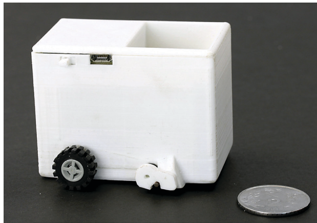
→ Sustainabot: a mini robot that prints using everyday grains and foodstuffs.
