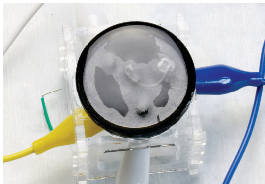
→ Liquid metal as a programmable material for visual and tactile output.
