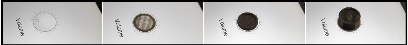
Figure 1. The Emergeables concept: instead of graphical widgets, tangible continuous controls emerge from the surface of the mobile device.
