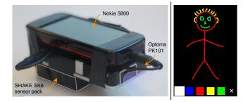
Figure 2. Our current prototype. Each user holds the device (left) in-hand, sketching on the screen (right) and moving to animate their projected story. Movements are recorded by the attached sensor pack.
