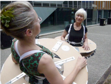
Figure 2. hipDisk exploits changing relationships between torso and hip to actuate sound.
