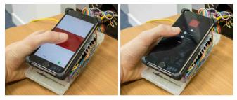
Figure 7. The GUI displayed on the phone. On the left is the menu to select the initial colour. On the right we see the chosen colour now in the centre pot, which activates the gel in that area on the back of the device.
