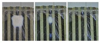
Figure 6. Hydrogel states as temperature is changed, Left: The gel is at its hardest, feeling like an oil-based paint. Centre: The gel is softer and thinned out, feeling more like an acrylic-based paint. Right: The gel is now at its softest after being fully thinned out, and feels more like a water-based paint.
