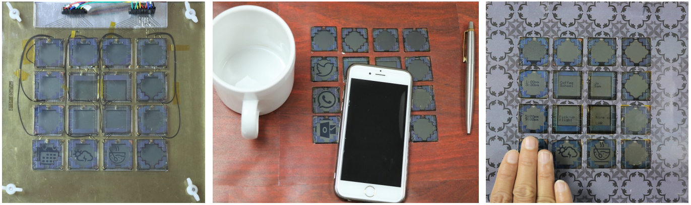
Figure 7. Left: our demonstrator PV-Tile prototype. Sixteen OPV cells are organised into a 4 \times 4 array. Digital displays are visible beneath the tiles (see icons in bottom row). Other images show the PV-Tile in simulated interaction contexts. Centre: a tabletop scenario, with displayed elements moving when occluded (see Fig. 6, row 1, images a and b). Right: a kitchen scenario, using shadow gestures to select and scroll through content (Fig. 6, row 4).
