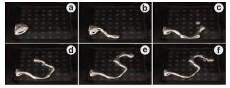
Figure 4. Process of drawing a letter "S" with EGaIn
