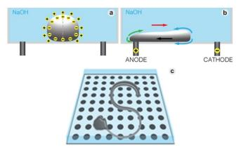
**Figure 1.** Liquid Metal Motion Mechanism: (a) Normal state without voltage (b) Deformation with positively applied voltage (c) Liquid Metal Control by Electrode Array
