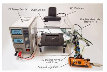
**Figure 2.** We use a 49 channel PWM driver controlled by an Arduino microcontroller to affect the voltages of the 7x7 graphite electrode array. The position and shape of liquid metal is tracked by a HD Web camera set up over the display surface.
