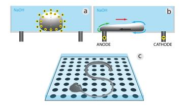
Figure 2. How the electric field creates deformation (a) A liquid metal blob far from the electrodes and in absence of field is subject to no force (b) Deformation occurs when the blob is in contact with one of the electrodes and an electric voltage is applied across it. (c) Deformation in this work as a 2D process.
