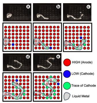
Figure 6. Basic electrode array control algorithm to make alphabet letter "S".
