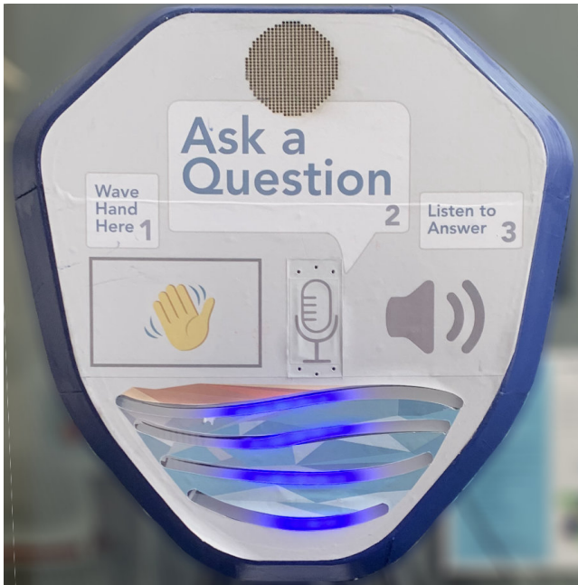
Figure 7: The SpeechBox prototype. Waving at the device triggers an audio prompt (via the speaker, top) to verbally ask a question. After an answer is provided, the user waves left or right to give feedback on the response’s accuracy. LED strips at the bottom provide wave and status feedback.
