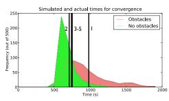
Figure 3. The simulator predicted times for convergence (from 500 runs) compared with the actual measured times (marked with vertical lines). The actual times fall well within the predicted times. Trials 3–5 are bunched very closely together. The long tails in the obstacle case are due to agents becoming stuck due to limited pathfinding ability.
