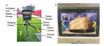
Figure 4: a) Final construction of the finished Lookout rig. b) Snapshot of a user viewing the Arena with their picture shown utilising the moustache filter.
